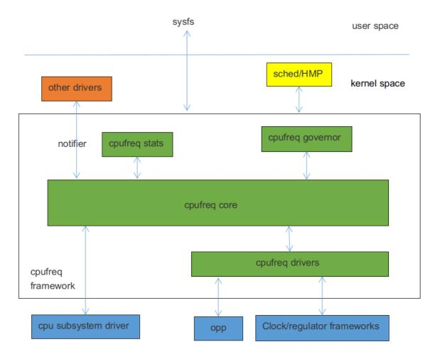
CPUFreq governor: It is used to determine when to chang the CPU frequency and which frequency will be chang to. The kernel includes the following governor:
