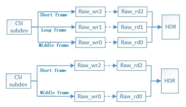
The CSI subdev obtains the output information of the sensor driver in multiple pad formats through get\_fmt, which corresponds to the source pad of the CSI.
