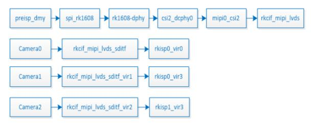
The dts configuration of RK1608 is mainly on the rk1608-dpy device node, which mainly includes input and output channels and resolution, as follows:
